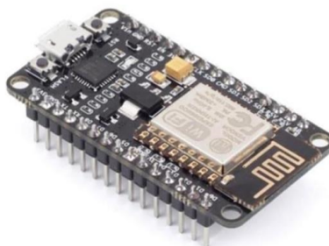
(The picture shows the ESP8266 NodeMCU WiFi module-plate)
